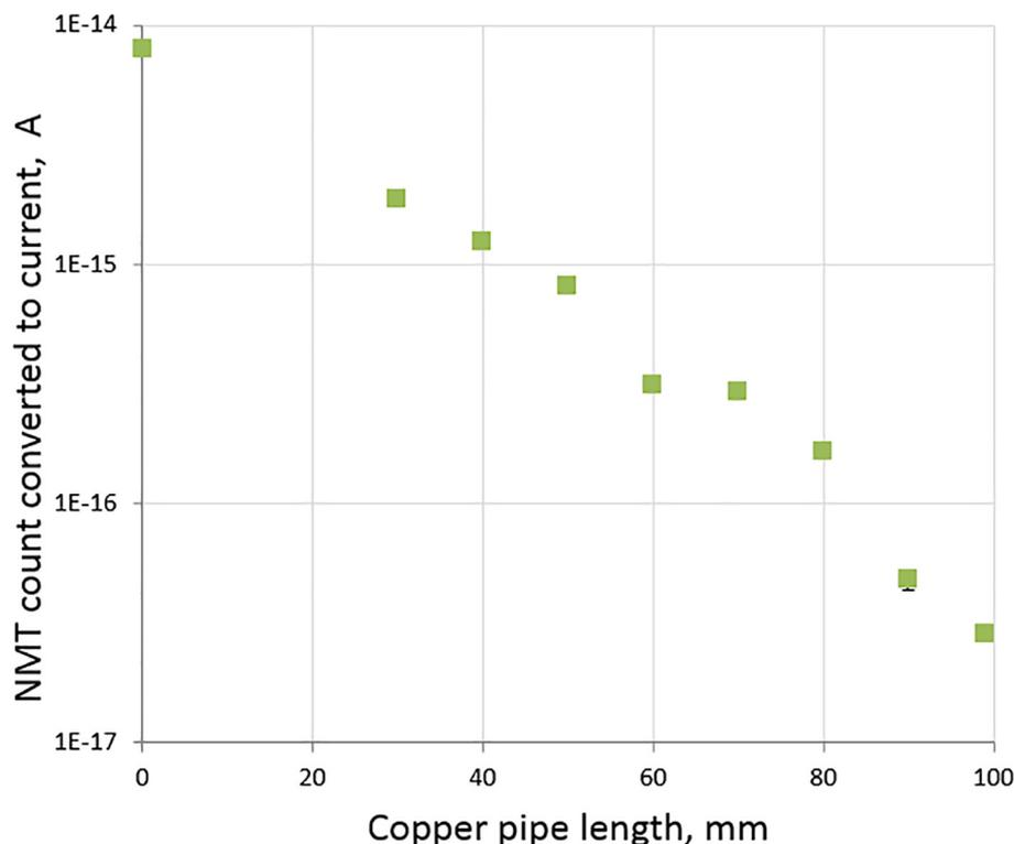
**Fig. 5.** Effective electric current data from the NMT ion counter vs. the copper tube length. Green squares represent the count occurring when  $^{241}\text{Am}$  radiation source present. The error bars for the green squares are smaller than the size of the squares. (For interpretation of the references to colour in this figure legend, the reader is referred to the web version of this article.)
