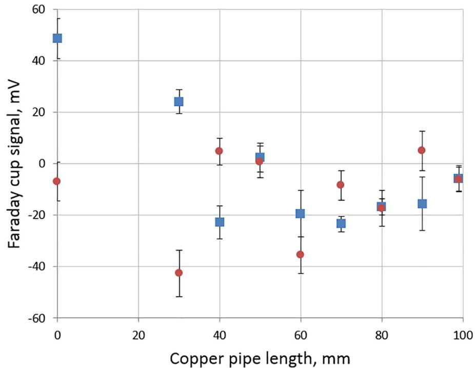
**Fig. 4.** Data from the electrometer based on the Faraday cup vs. the copper tube length. Blue squares represent the count occurring when the  $^{241}\text{Am}$  radiation source is present, red circles for when the  $^{241}\text{Am}$  radiation source was absent. The errors bars represent the standard deviation of 9 measurements using the electrometer. (For interpretation of the references to colour in this figure legend, the reader is referred to the web version of this article.)
