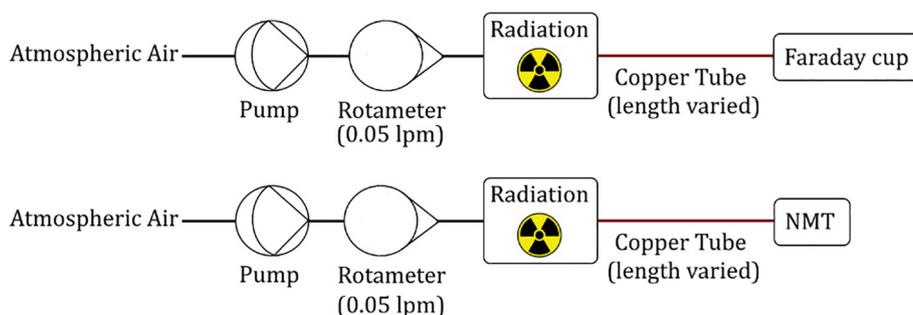
Fig. 2. Schematic of the set-up for the comparison of the NMT and Faraday cup based electrometer detection of ion concentrations in the same flow. The “radiation” rectangle indicates the ionization chamber with  $^{241}\text{Am}$ .
